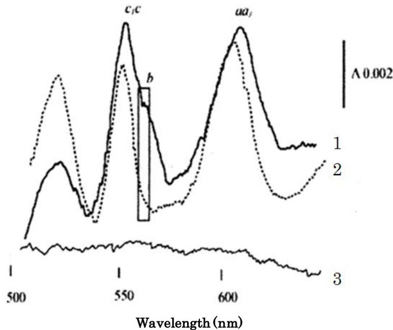
Fig.5 Reduced-minus oxidized difference spectrum measured using SMP in absence and presence of  $\text{AgNO}_3$ .
