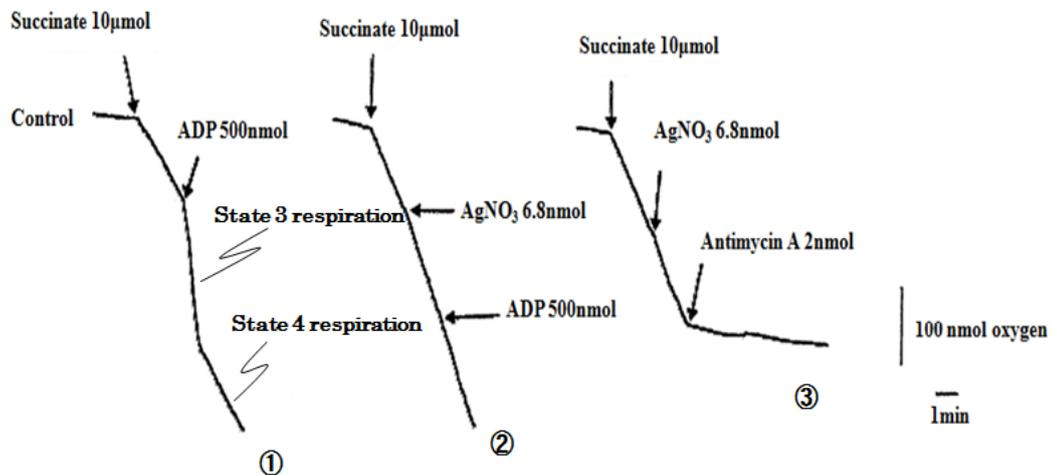
Fig.3 the effect of  $\text{AgNO}_3$  on the FAD-linked respiration oxidizing succinate. Typical oxygraph data measured by use of an oxygen electrode. The reaction medium was composed of 0.25M sucrose, 5mM magnesium nitrate, 5mM inorganic phosphate, 10mM Tris-nitrate, 0.5mM EDTA and ca 1mg mitochondrial protein in a final volume of 2.0ml (pH 7.4). The reaction was performed at 30°C and was initiated by adding a substrate(succinate).
